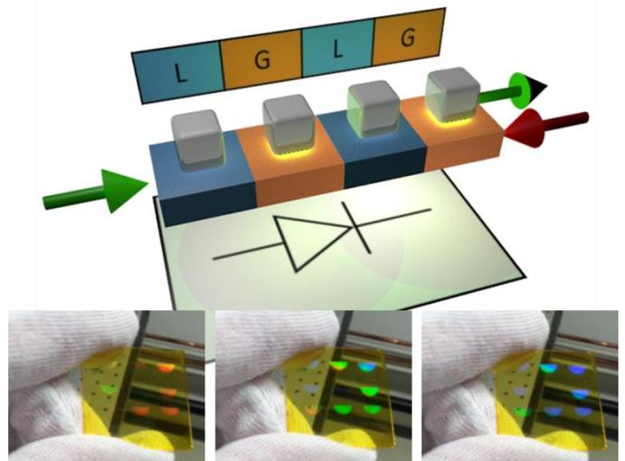
**Schematic of the anticipated “optical diode” in analogy to the flow of an electrical current in a diode and a first approach to this device from the König group.**
